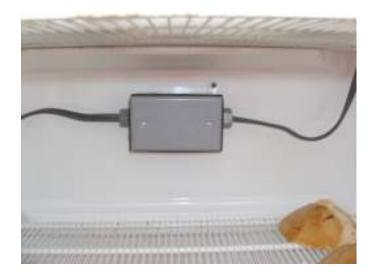
IF YOU ARE FAMILIAR WITH ELECTRICAL WIREING, A PROFESSIONAL CONTRACTOR WILL NOT BE NEEDED. LOCATE WHERE YOU WILL EXIT YOUR SHOP FOR THE ELECTRIC SUPPLY TO YOUR KILN. IF AN OUTSIDE RECEPTACLE IS AVAILABLE BE SURE IT IS A GFI CIRCUIT. MOUNT WATER TIGHT ELECTRICAL BOXES, ONE ON THE OUTSIDE OF THE KILN FOR A ON/OFF SWITCH, ONE ON THE INSIDE TOP FOR A THERMASTAT AND ONE ON THE BOTTOM FOR A HOODED LAMP. UF WIREING AND WATER TIGHT CONNECTORS ARE NEEDED THROUGH OUT THE INSTALLATION FOR SAFTY.
