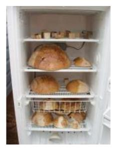
A BOWL DRYING KILN CAN BE MADE FROM MOST ANY INSULATED ENCLOSURE WHERE AIR FLOW AND TEMPERTURE IS CONTROLLED. DISCARDED UPRIGHT REFRIGERATORS AND FREEZERS ARE ONE OF THE EASIEST TO BUILD. USUALLY THEY CAN BE AVAILABLE FOR LITTLE OR NO COST FROM AN APPLIANCE REPAIR CENTER.
