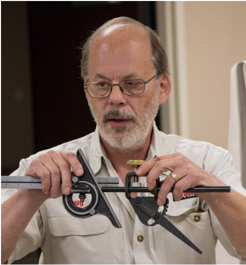
(left) Doug shows how to measure grind angle with a combination square
