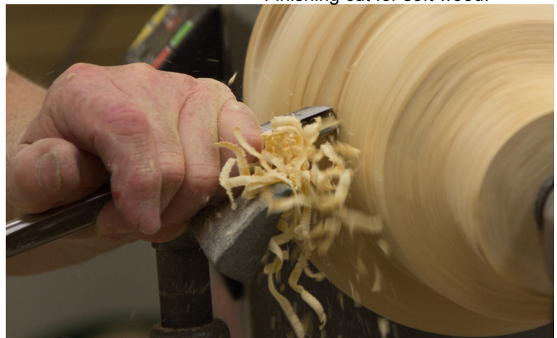
Finishing cut in action
