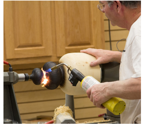
Finishing with a torch
